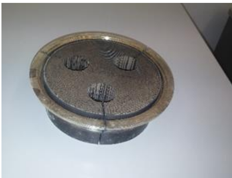
Figure 95: Part of the Pd-Pt/CZ catalyst after operation at gas engine. Samples were drilled out with diameter of 25mm and length of 42mm.
