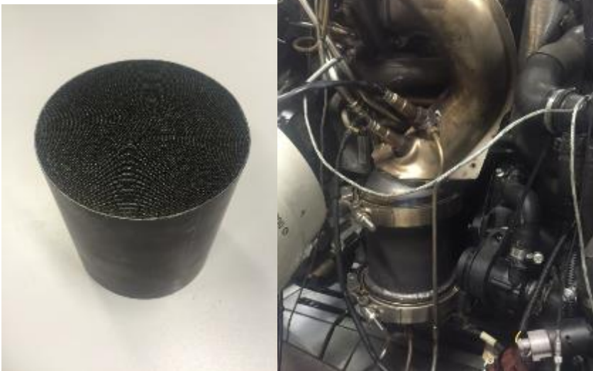
Figure 91: Left: FVV/KIT sample. Right: Placement of sample at test-engine.
