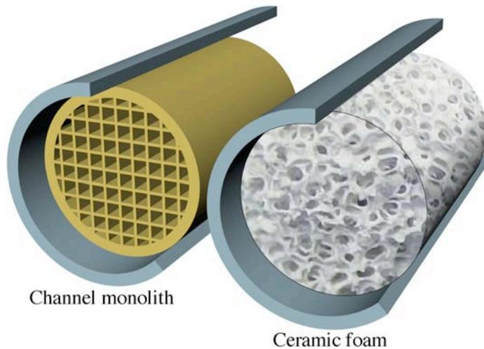
Figure 3: Catalysts inside the tubes may be supported on channel-monolith or ceramic-foam structures.
