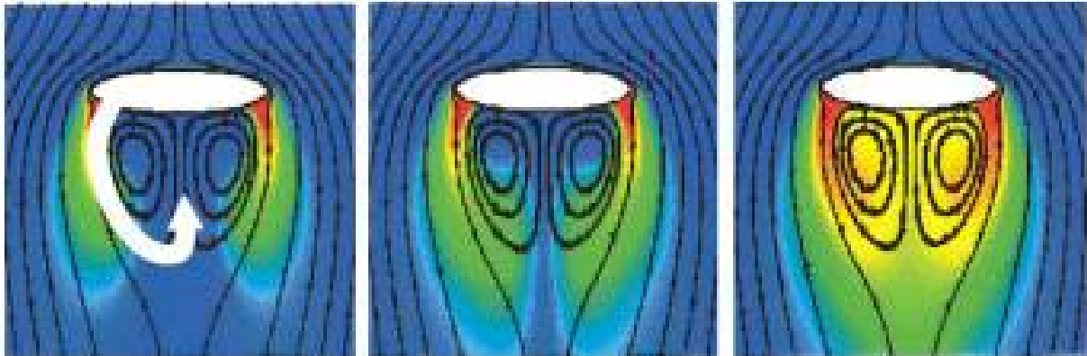
Figure 10: Snapshots of the computed developing concentration of the product in the wake of a bubble in a gas-liquid-solid reaction; taken from Raffensberger et al. [122] .
