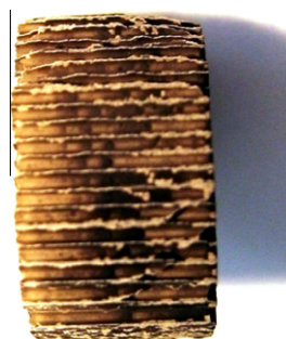
Fig. 13. Photo taken from a catalytic monolith removed from the reactor after operation C/O = 1.2. The inlet flow enters the catalyst from the left side.
