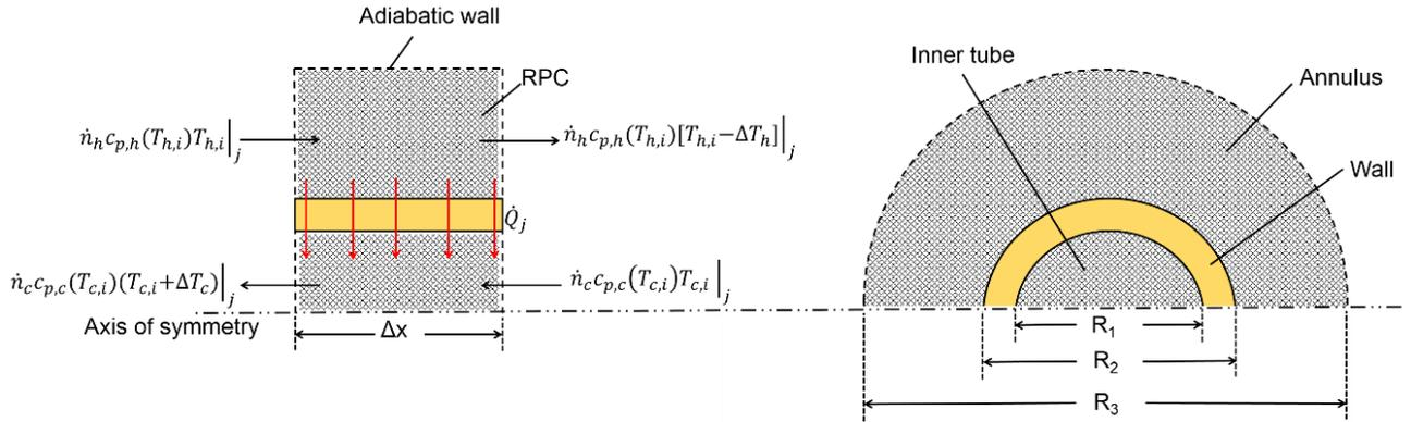
**Figure 3.3 Energy flows in a finite volume element 'j' of the HX.**
