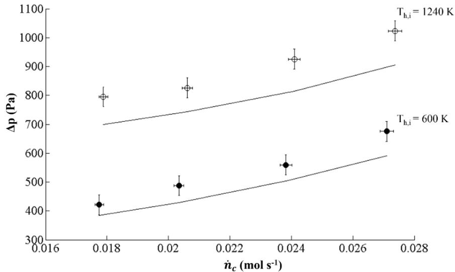
**Figure 4.10 Pressure drop across the heat exchanger as a function of cold stream molar flow rate. The open symbols are for  $T_{h,i} = 1240$  K and the closed symbols are for  $T_{h,i} = 600$  K. The solid lines represent the predicted values.**
