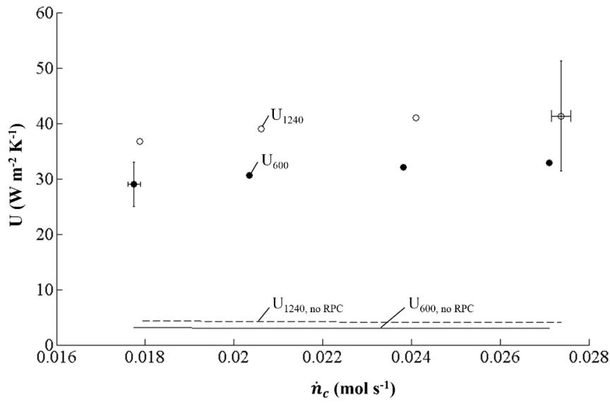
**Figure 4.6 Overall heat transfer coefficient as a function of cold gas molar flow rate. The open symbols are for  $T_{h,i} = 1240$  K and the closed symbols are for  $T_{h,i} = 600$  K. The uncertainties are reported for a 95% confidence interval. The dashed line is for HX without RPC at  $T_{h,i} = 1240$  K and the solid line is for HX without RPC at  $T_{h,i} = 600$  K.**
