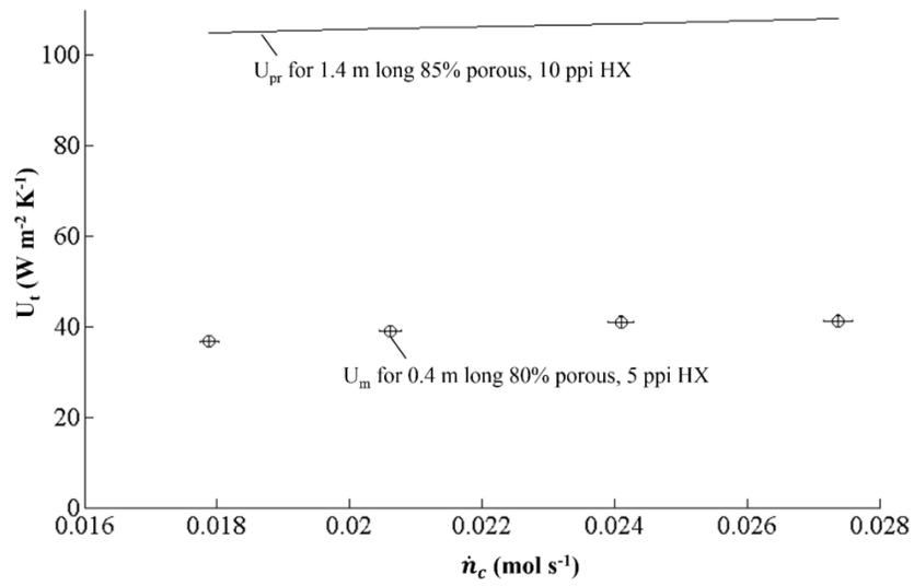
**Figure 4.12 Overall heat transfer coefficient of the heat exchanger as a function of cold stream molar flow rate. The open symbols are for experiments run at  $T_{h,i} = 1240$  K. The solid line represents the predicted values from the 1-D model.**
