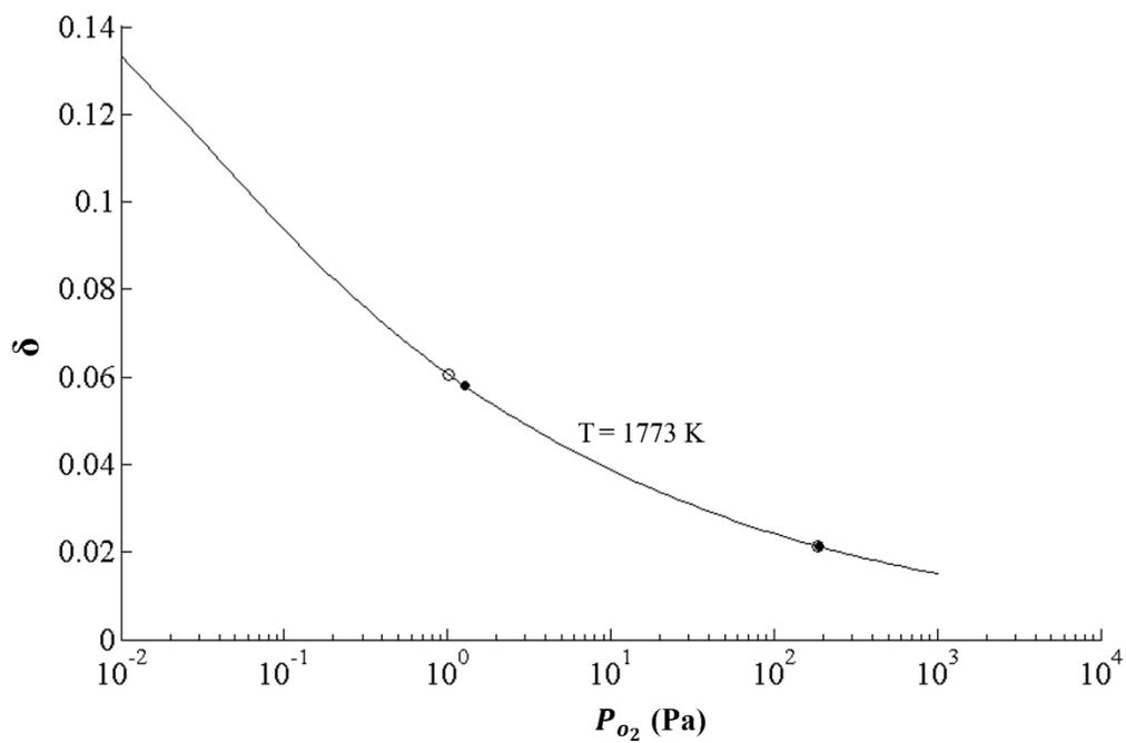
**Figure C.1** Variation of ceria non-stoichiometry,  $\delta$ , with partial pressure of oxygen,  $P_{O_2}$ . The open symbols are the baseline values at  $P_{\text{tot}} = 1 \times 10^5 \text{ Pa}$  and the closed symbols are the values at elevated ceria bed pressures of  $1.28 \times 10^5 \text{ Pa}$  during reduction and  $1.06 \times 10^5 \text{ Pa}$  during oxidation.
