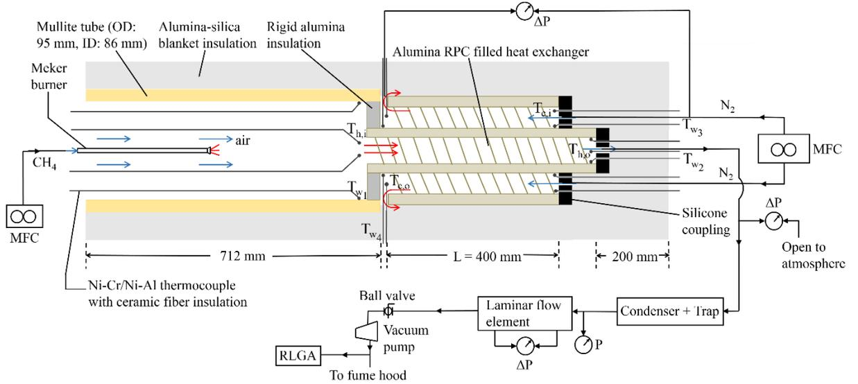
**Figure 4.4 Cross-section of experimental apparatus to measure  $U$ ,  $\varepsilon$  and  $\Delta p$  of the heat exchanger prototype. Thermocouple locations are shown with grey dots. The arrows indicate direction of gas flow. RLGGA = Raman Laser Gas Analyzer**
