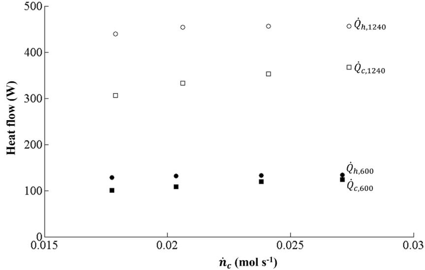
**Figure 4.9 Heat flow as a function of cold stream molar flow rate. The open symbols indicate experiments run at  $T_{h,i} = 1240 \text{ K}$  and the closed symbols indicate experiments run at  $T_{h,i} = 600 \text{ K}$ .**
