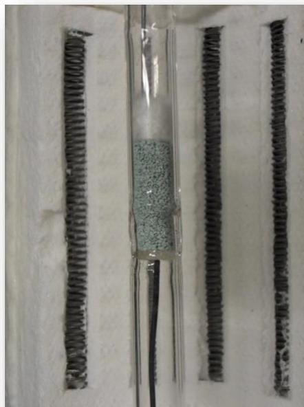
**Figure 3.2** Schematic drawing of the fixed bed reactor (a) and picture of the real catalytic bed (b).
