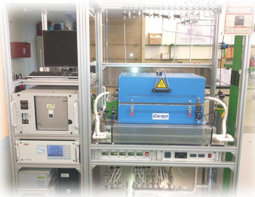
Tests of catalyst powders ( $d = 0,5$  cm) and catalyst coated honeycombs ( $d = 2 - 2.54$  cm, length < 4 cm)
