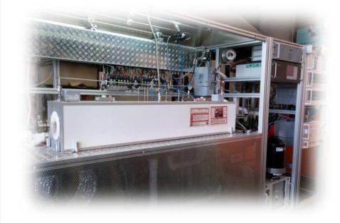
Tests of catalyst coated honeycombs (d = 2.54 cm, length < 15 cm)
