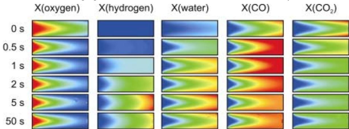
Fig. 2. Gas-phase mole fractions in a single channel in the centre of the monolith during light-off; the radial coordinates is stretched. (ranges: O<sub>2</sub> = 0 - 0.08, H<sub>2</sub> = 0 - 0.05, H<sub>2</sub>O = 0 - 0.07, CO = 0 - 0.05, CO<sub>2</sub> = 0 - 0.03)
