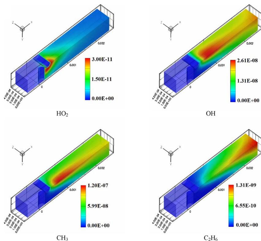
Fig. 5. Numerically predicted contour profiles of mole fractions of radical species ( $\text{HO}_2$ ,  $\text{HO}$ , and  $\text{CH}_3$ ) and stable products ( $\text{C}_2\text{H}_6$ ). Conditions:  $\text{CH}_4/\text{O}_2$  vol. ratio = 2.5, axial inlet flow velocity = 10 m/s, inlet temperature = 600 K, and pressure = 1.3 bar. For visual clarity the orientation of the flow direction is opposite from the one in Figs. 1 and 4.
