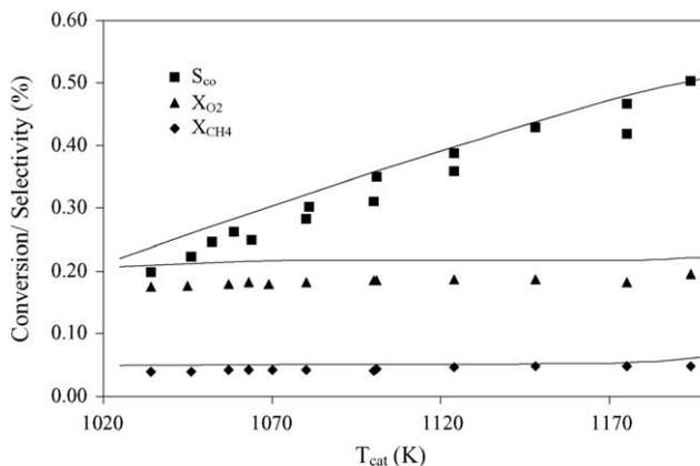
Fig. 3. Comparison of experimental data (symbols) and predicted methane and oxygen conversion ( $X$ ) and CO selectivity ( $S$ ) as function of catalyst temperature. Conditions: CH<sub>4</sub>/O<sub>2</sub> vol. ratio = 2.5, axial inlet flow velocity = 10 m/s, inlet temperature = 600 K, and pressure = 1.3 bar.
