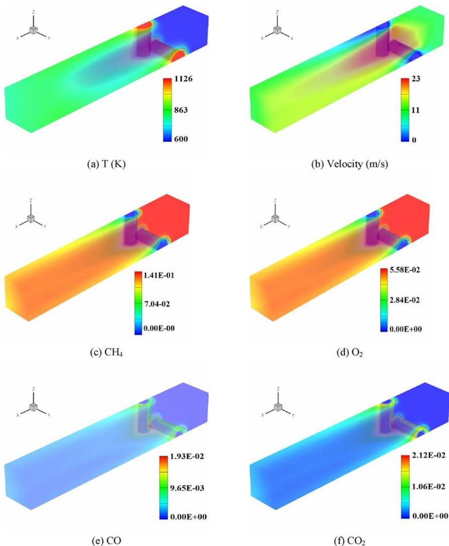
Fig. 4. Numerically predicted contour profiles of temperature, magnitude of velocity, and mole fractions of the major species. Conditions: CH<sub>4</sub>/O<sub>2</sub> vol. ratio = 2.5, axial inlet flow velocity = 10 m/s, inlet temperature = 600 K, and pressure = 1.3 bar.
