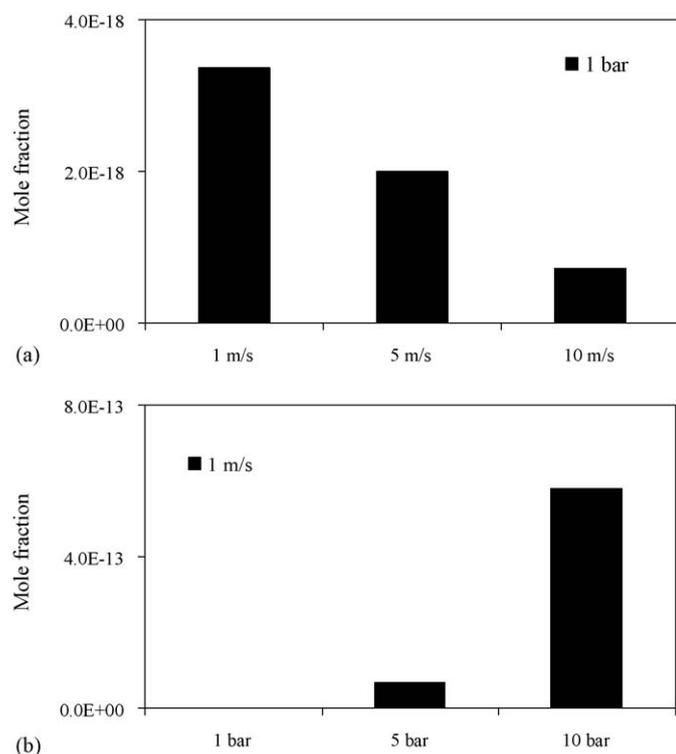
Fig. 6. Impact of (a) inlet gas velocity at 1 bar and (b) total pressure at 1 m/s on the outlet concentration of C<sub>2</sub>H<sub>6</sub>. Conditions: CH<sub>4</sub>/O<sub>2</sub> vol. ratio = 2.5, inlet temperature = 600 K.
