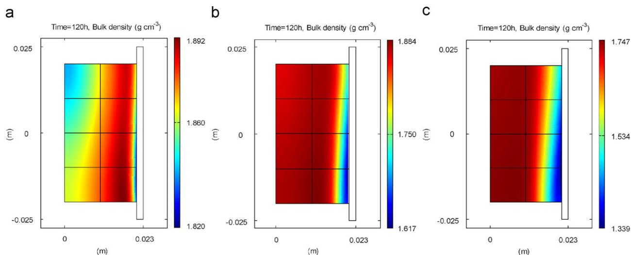
Fig. 5. The predicted bulk density distributions (120h densification) corresponding to feed gas of (a) 20 kPa  $\text{CH}_4$ , (b) 20 kPa  $\text{CH}_4$  with 4 kPa additional  $\text{H}_2$  and (c) 20 kPa  $\text{CH}_4$  with 10 kPa additional  $\text{H}_2$ .
