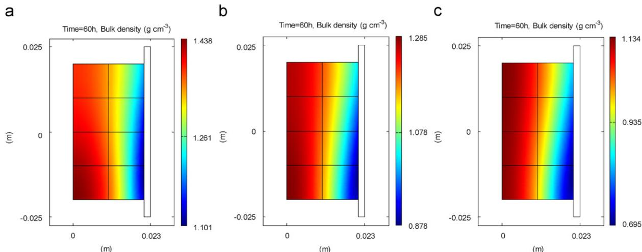
Fig. 6. The predicted bulk density distributions (60h densification) corresponding to feed gas of (a) 20 kPa  $\text{CH}_4$ , (b) 20 kPa  $\text{CH}_4$  with 4 kPa additional  $\text{H}_2$  and (c) 20 kPa  $\text{CH}_4$  with 10 kPa additional  $\text{H}_2$ .
