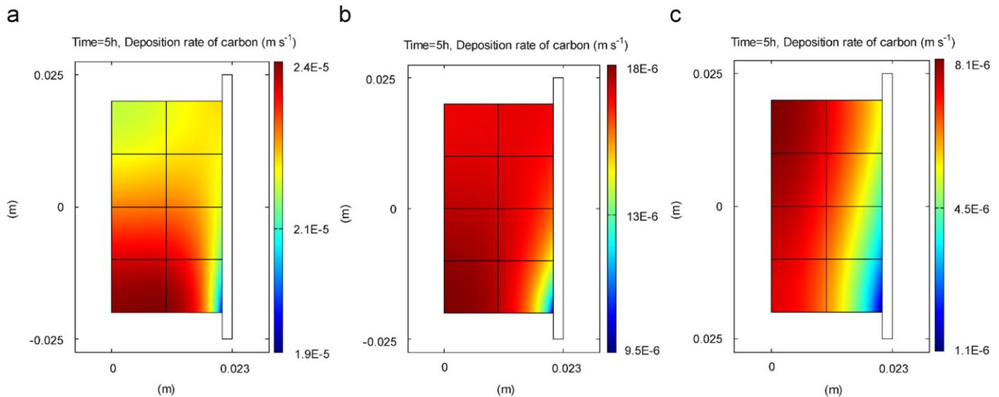
Fig. 8. The local deposition rate of carbon from (a, b) acetylene and (c) benzene, corresponding to feed gas of (a) pure methane, (b) CH<sub>4</sub> with 4 kPa additional H<sub>2</sub> and (c) CH<sub>4</sub> with 10 kPa additional H<sub>2</sub>.
