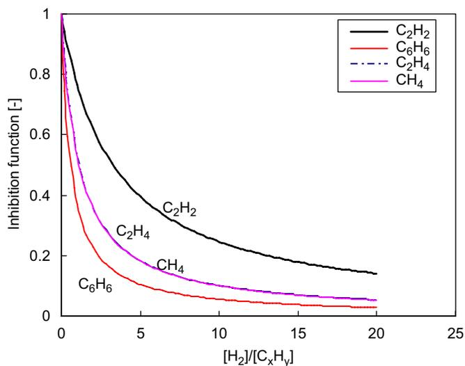
Fig. 2. Inhibition functions of various hydrocarbons (profile of CH<sub>4</sub> at 1373 K, others at 1273 K) as a function of the hydrogen content.
