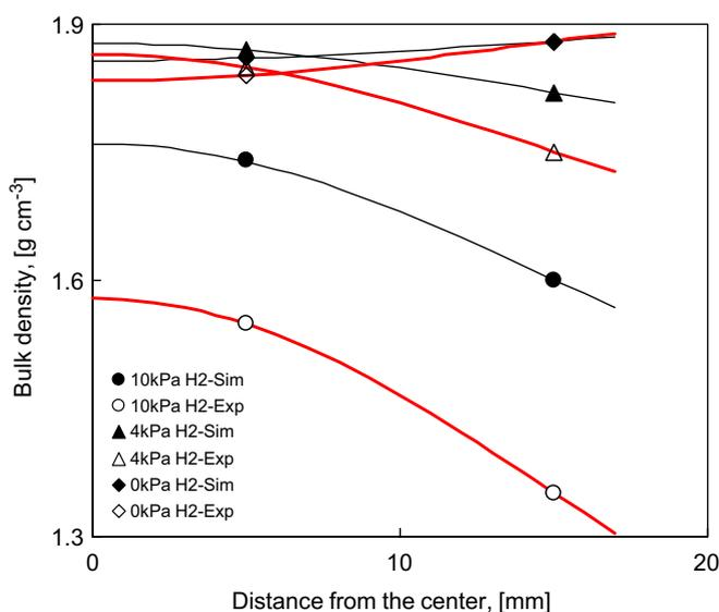
Fig. 7. Bulk density distributions after 120h densification.
