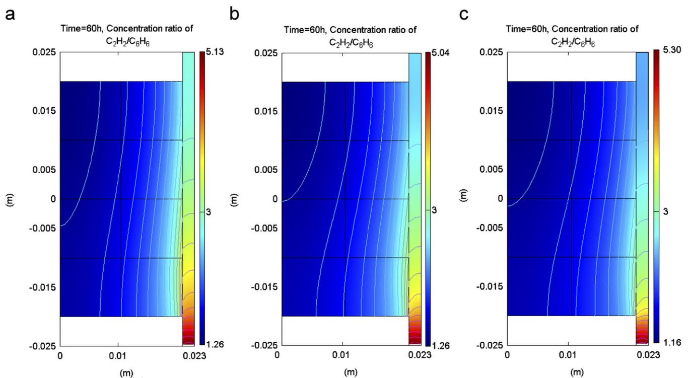
Fig. 9. The concentration ratio of acetylene to benzene corresponding to feed gas of (a) pure methane, (b) CH<sub>4</sub> with 4 kPa additional H<sub>2</sub> and (c) CH<sub>4</sub> with 10 kPa additional H<sub>2</sub>.
