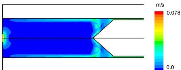
Fig. 5. Simulated flow field from the bottom of the reactor to the in-situ sampling apparatus (Flow rate at the inlet: 0.059 m/s).
