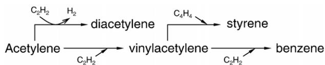
Fig. 8. The sketch of reaction flow in acetylene pyrolysis.
