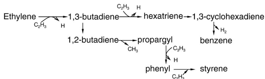
Fig. 9. The sketch of reaction flow in ethylene pyrolysis.
