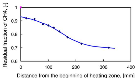
Fig. 6. Residual fraction of methane as a function of the distance from the beginning of the heating zone (error limit:  $\pm 0.19\%$ ).
