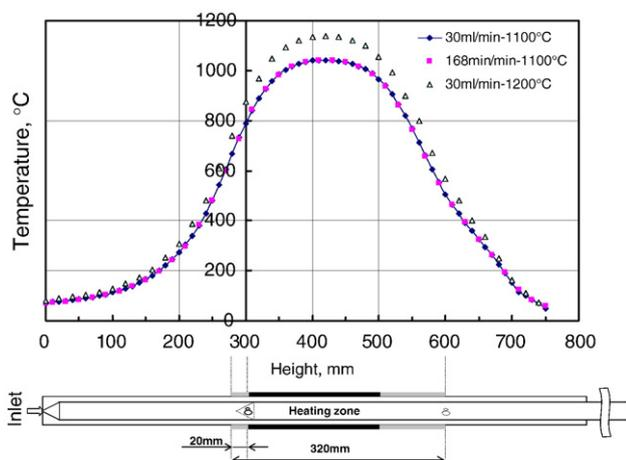
Fig. 3. Temperature profiles of the reactor measured for the empty tube.
