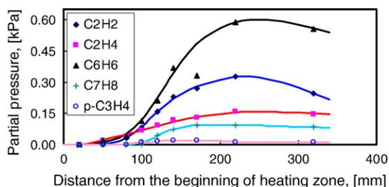
Fig. 7. Partial pressures of intermediate species in methane pyrolysis (error limits,  $C_2H_2$ : -4.1%,  $C_2H_4$ : -2.4%,  $C_6H_6$ : 10.8%,  $C_7H_8$ : 12.2% and  $p-C_3H_4$ : -11.5%).
