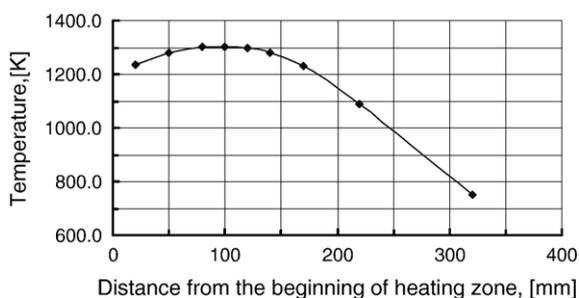
Fig. 4. Temperature distribution in the tubular reactor measured using the thermal couple of the in-situ sampling device.
