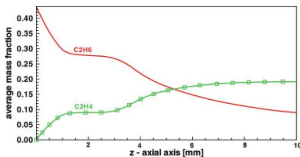
**Figure 9. Average mass fraction profiles of  $\text{C}_2\text{H}_6$  and  $\text{C}_2\text{H}_4$  with the optimal setting.**
