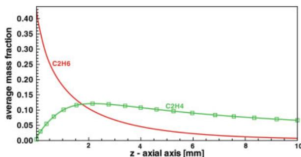
**Figure 8. Average mass fraction profiles of  $\text{C}_2\text{H}_6$  and  $\text{C}_2\text{H}_4$  with the initial setting.**
