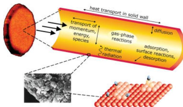
**Figure 1. Processes occurring in a catalytic monolith operated at high temperature.**
