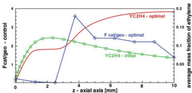
**Figure 7.  $F_{\text{cat/geo}}(z)$  profile and the average mass fraction of  $\text{C}_2\text{H}_4$  at the initial and at optimal solutions.**
