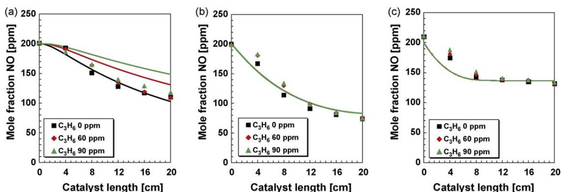
Fig. 4. Influence of C<sub>3</sub>H<sub>6</sub> concentration on the NO oxidation on Pt/Al<sub>2</sub>O<sub>3</sub> under steady-state lean conditions at various temperatures; comparison of experiment (□, ◇, △) and simulation (—), gas composition: 200 ppm NO, 0.04 vol.% CO, 12 vol.% O<sub>2</sub>, 7 vol.% CO<sub>2</sub>, 10 vol.% H<sub>2</sub>O, balance N<sub>2</sub>. (a) 250 °C; (b) 350 °C; (c) 450 °C.
