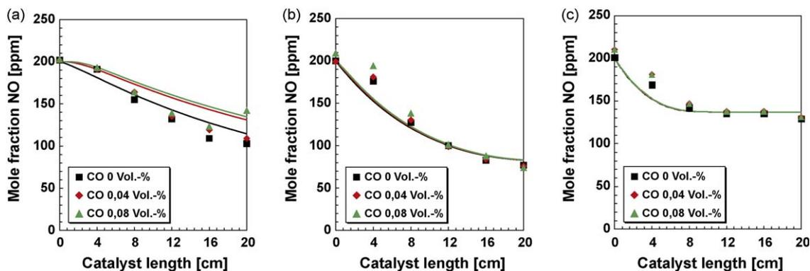
Fig. 3. Influence of CO concentration on the NO oxidation on Pt/Al<sub>2</sub>O<sub>3</sub> under steady-state lean conditions at various temperatures; comparison of experiment (□, ◇, △) and simulation (—), gas composition: 200 ppm NO, 60 ppm C<sub>3</sub>H<sub>6</sub>, 12 vol.% O<sub>2</sub>, 7 vol.% CO<sub>2</sub>, 10 vol.% H<sub>2</sub>O, balance N<sub>2</sub>. (a) 250 °C; (b) 350 °C; (c) 450 °C.
