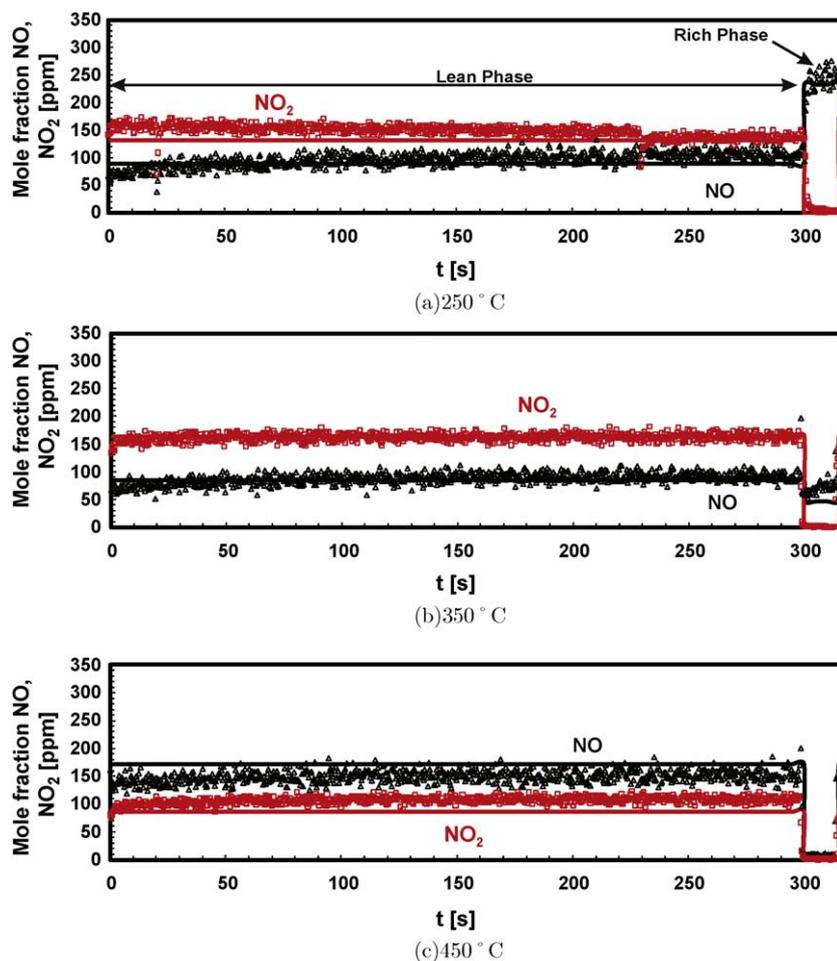
**Fig. 6.** Lean/rich cycle of 300 s/15 s on Pt/Al<sub>2</sub>O<sub>3</sub> at various temperatures; Comparison of experiment ( $\Delta$ ,  $\square$ ) and simulation (—), gas composition listed in Table 2. (a) 250 °C; (b) 350 °C; (c) 450 °C.
