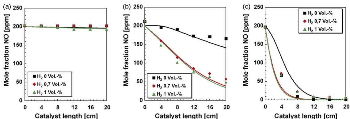
Fig. 5. Influence of H<sub>2</sub> concentration on the NO reduction on Pt/Pt/Al<sub>2</sub>O<sub>3</sub> under steady-state rich conditions at various temperatures; comparison of experiment (□, ◇, △) and simulation (—), gas composition: 200 ppm NO, 2.1 vol.% CO, 60 ppm C<sub>3</sub>H<sub>6</sub>, 0.9 vol.% O<sub>2</sub>, 7 vol.% CO<sub>2</sub>, 10 vol.% H<sub>2</sub>O, balance N<sub>2</sub>. (a) 250 °C; (b) 350 °C; (c) 450 °C.
