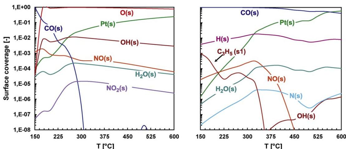
**Fig. 2.** Simulated surface coverages (logarithmic scale) on platinum at steady-state conditions as a function of temperature, values taken at channel outlet; lean phase (left), rich phase (right), gas composition listed in Table 2.
