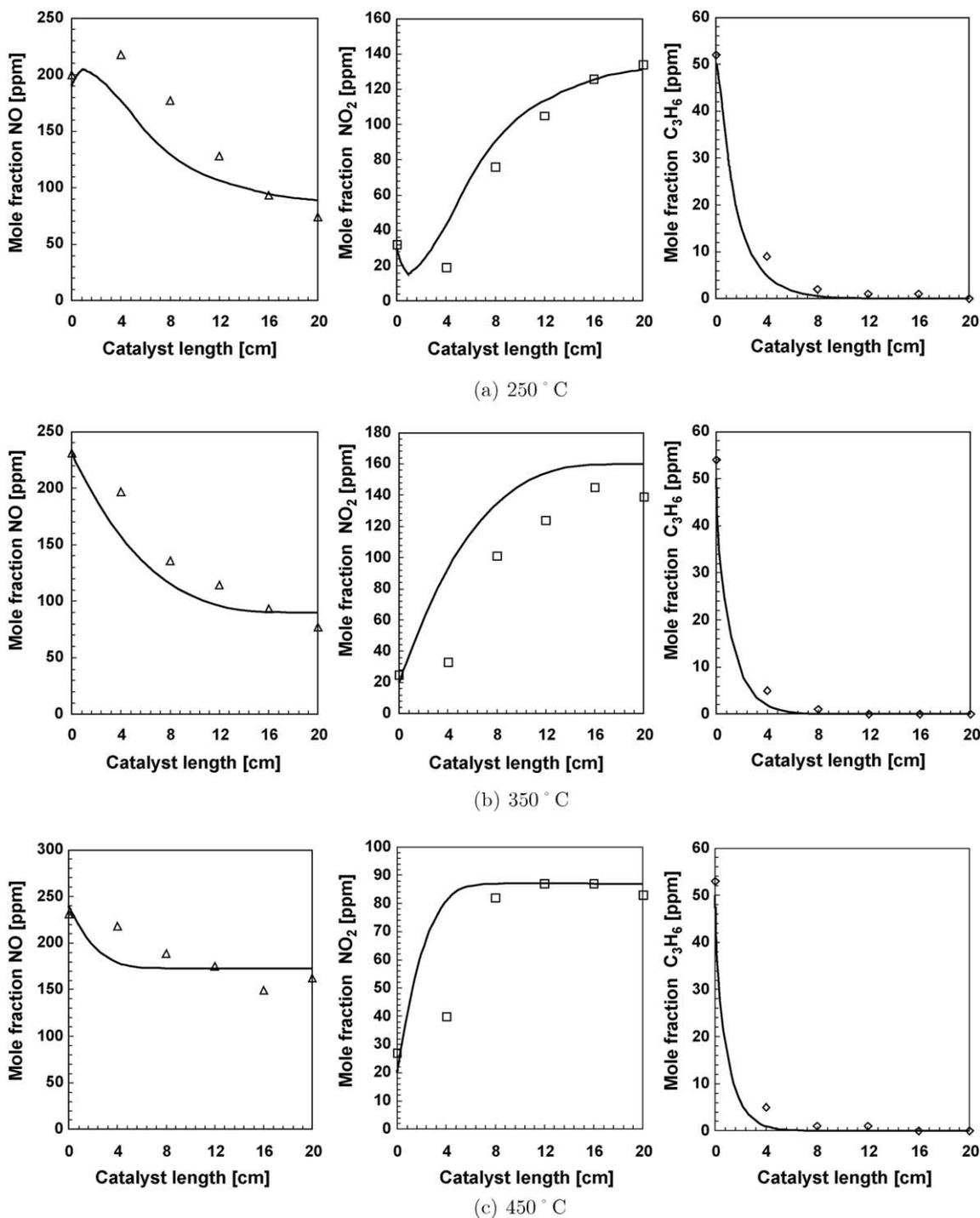
Fig. 7. Axial profiles of NO, NO<sub>2</sub> and C<sub>3</sub>H<sub>6</sub> during the lean phase of lean/rich cycling at various temperatures; comparison of experiment (Δ, □, ◇) and simulation (—). (a) 250 °C; (b) 350 °C; (c) 450 °C.
