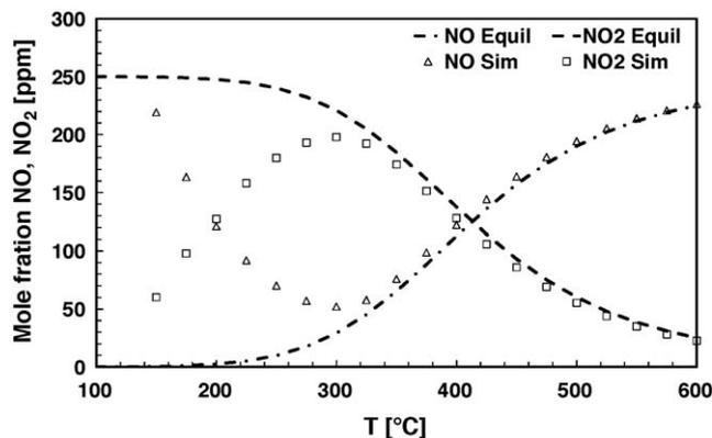
Fig. 1. Comparison of the thermodynamic equilibrium concentrations (–) and simulated concentrations of NO ( $\Delta$ ) and  $NO_2$  ( $\square$ ) as a function of temperature (250 ppm NO, 12 vol.%  $O_2$  in Argon).
