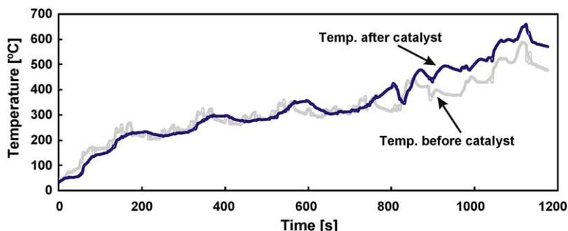
**Fig. 8.** Measured temperature before (in front of) and after (behind) the Pt/Al<sub>2</sub>O<sub>3</sub> catalyst during NEDC as a function of time, cushioned temperature ramp due to additional uncoated monolith prior to the platinum catalyst.
