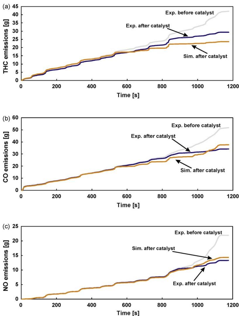
**Fig. 9.** Cumulative emissions of (a) THC, (b) CO and (c) NO of a commercial Pt/Al<sub>2</sub>O<sub>3</sub> catalyst during NEDC as a function of time; comparison of experimental and simulated data.
