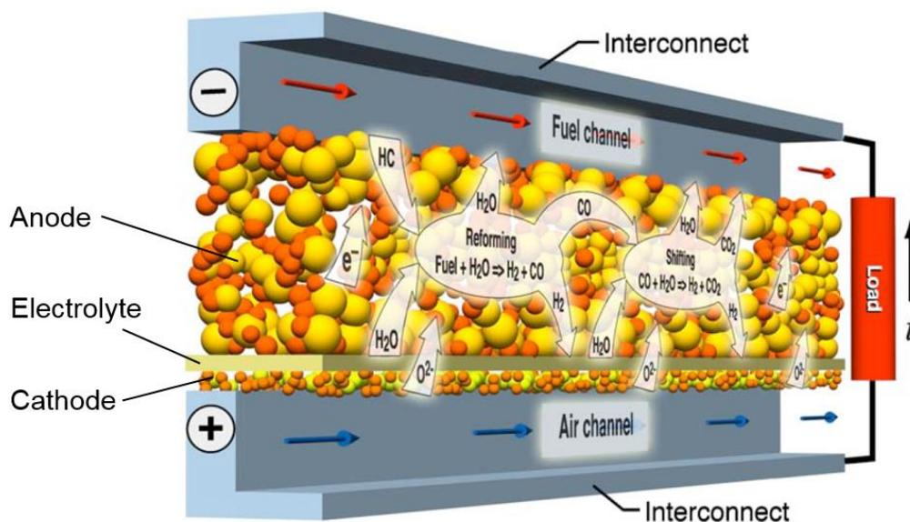
Abbildung 1: Schematic representation of a DIR-SOFC
