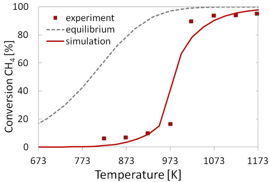
**Figure 4.48** Effect of the reaction temperature on conversion of  $\text{CH}_4$  over pre-calcined  $\text{Ni}/\text{Al}_2\text{O}_3$ ,  $\text{CH}_4/\text{O}_2=1.78$ , 1 bar;  $T_{\text{range}}=673\text{-}1173\text{ K}$ ; total flow rate of  $50\text{ cm}^3/\text{min}$  [16].
