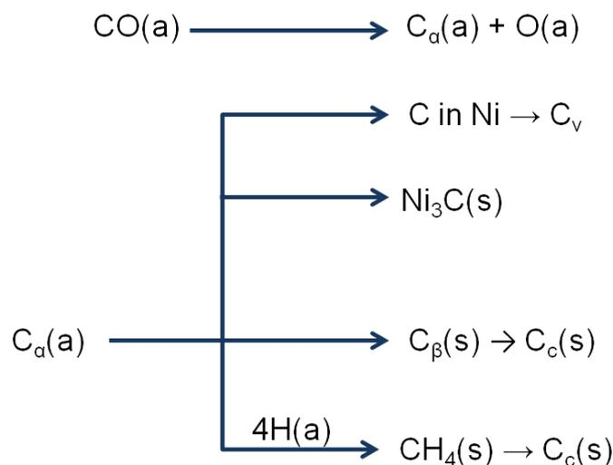
**Figure 5.9** Formation, transformation and gasification of carbon on nickel, as proposed by Bartholomew (a, g, s refer to adsorbed, gaseous and solid states, respectively) [276].
