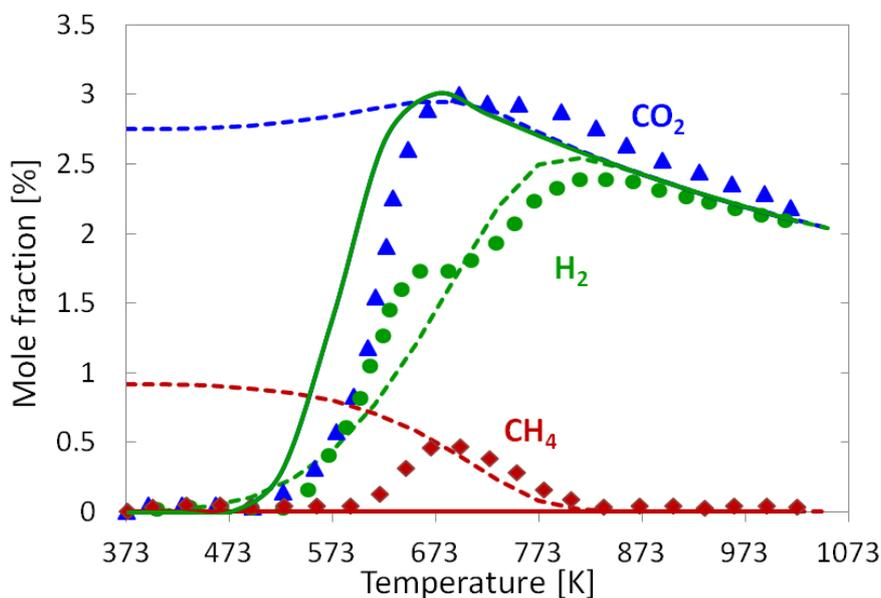
**Figure 4.22** Comparison of experimentally (symbols) and numerically predicted (lines) mole fractions as a function of temperature for WGS in a fixed bed reactor: **a)** CO and H<sub>2</sub>O; **b)** CO<sub>2</sub>, H<sub>2</sub>, and CH<sub>4</sub>, inlet gas composition of 3.6 vol.% CO, 4.3 vol. % H<sub>2</sub>O in N<sub>2</sub>; 1 bar;  $T_{inlet} = 373$  K; 4 SLPM; dashed lines = equilibrium composition at given temperature.
