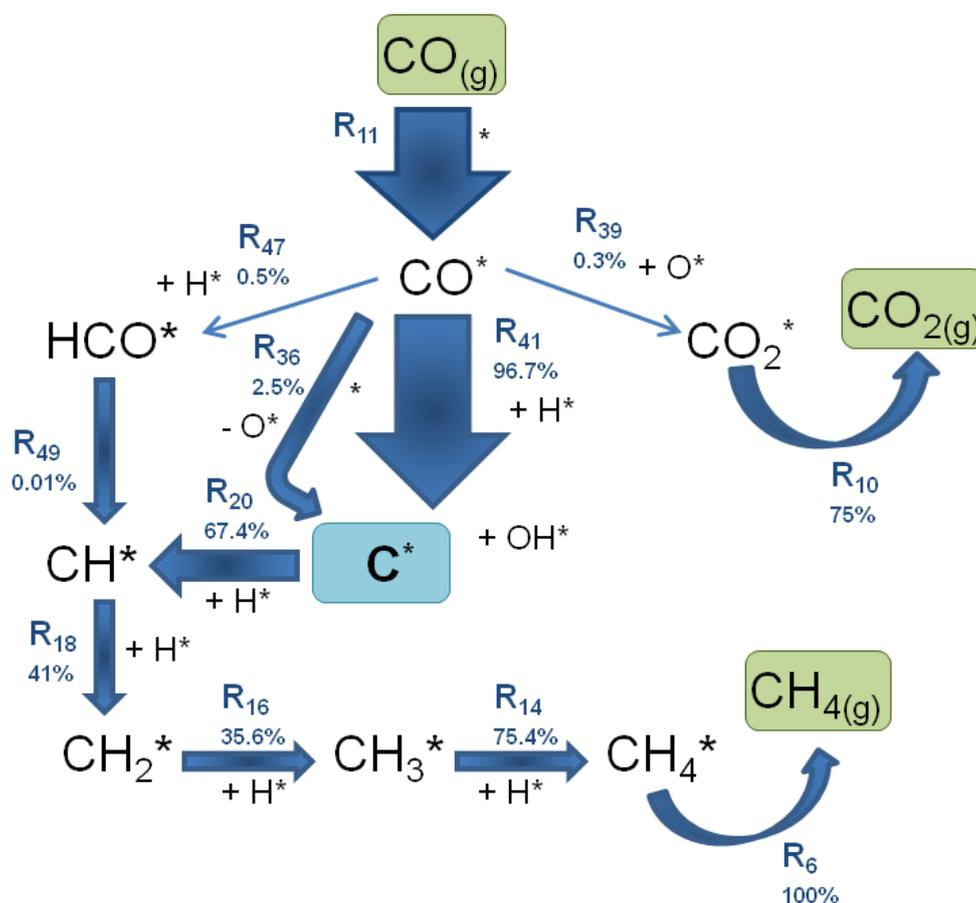
**Figure 5.6** Reaction flow analysis for CO methanation on nickel at 673K (400°C), 1bar, with an inlet mole composition of 2.0.vol% CO and 7.0.vol %  $\text{H}_2$  in  $\text{N}_2$  dilution.
