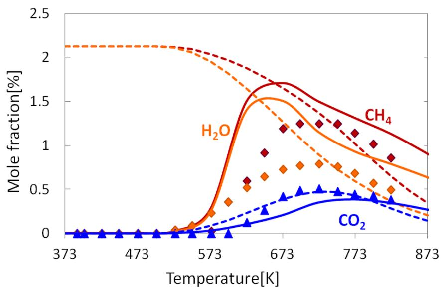
**Figure 5.7** Comparison of experimentally determined (symbols) and numerically predicted (lines) mole fractions as function of temperature for CO methanation: **a)** CO and H<sub>2</sub>; **b)** CO<sub>2</sub>, CH<sub>4</sub>, and H<sub>2</sub>O; inlet gas composition of = 2.04 vol.% CO and 7.0 vol.% H<sub>2</sub> in N<sub>2</sub> dilution; 1bar;  $T_{inlet}=373$  K; total flow rate of 4 SLPM; dashed lines =equilibrium composition at given temperature.
