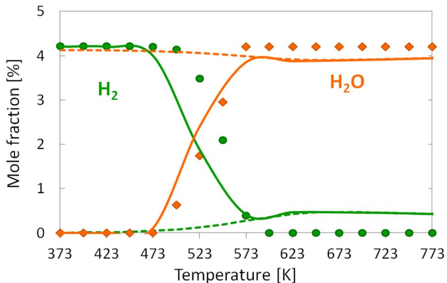
**Figure 4.17** Comparison of experimentally determined (symbols) and numerically predicted (lines) mole fractions as a function of temperature for preferential CO oxidation over a monolith catalyst: **a)** CO and CO<sub>2</sub>; **b)** H<sub>2</sub> and H<sub>2</sub>O; inlet gas composition of 4.3 vol.% CO, 4.2 vol.% H<sub>2</sub>, 4.0 vol.% O<sub>2</sub> in N<sub>2</sub>; 1 bar;  $T_{inlet} = 373$  K; total flow rate of 4 SLPM; dashed lines = equilibrium composition at given temperature.
