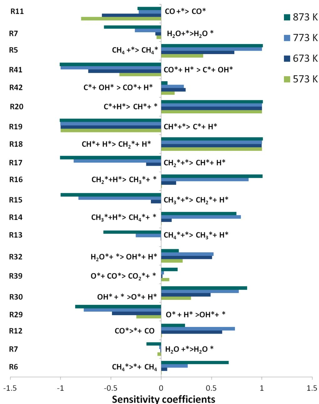
**Figure 5.1** Sensitivity analysis of  $\text{CH}_4$  gas-phase concentration for WGS reaction at different temperature points. Inlet gas composition is chose to be 3.6 vol.% CO, 4.3 vol.%  $\text{H}_2\text{O}$  in  $\text{N}_2$  dilution; 4 SLPM; at 1bar.
