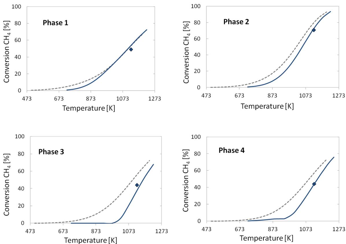
**Figure 4.59** Comparison of the experimental and numerical results for methane conversion as a function of temperature, Phase 1- 9, 20 bar; symbols = experiment, lines = simulation, dashed lines = equilibrium composition.
