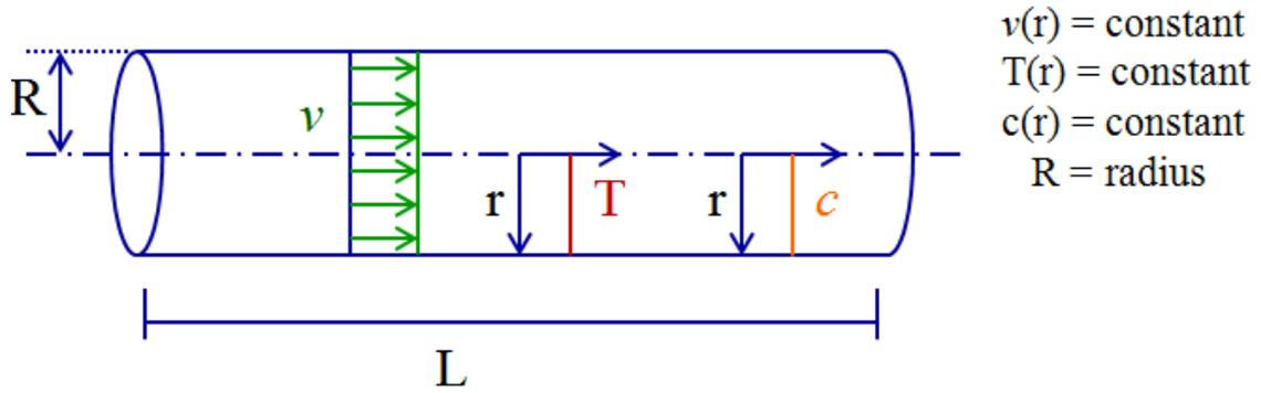
**Figure 2.3** Schematic diagram of a plug-flow reactor
