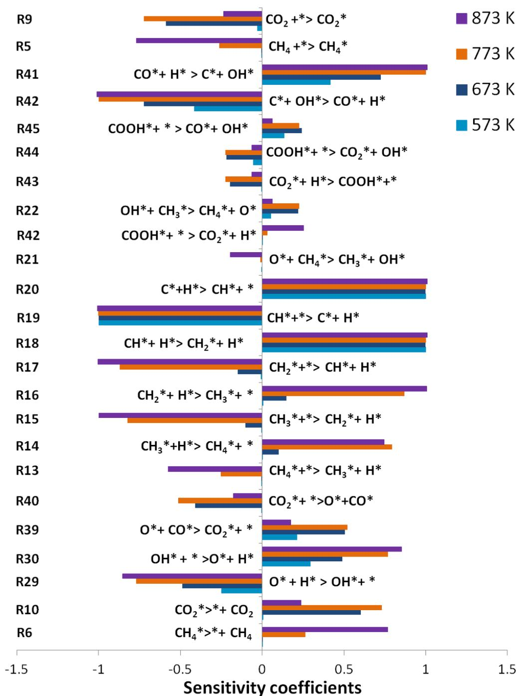
**Figure 5.3** Sensitivity analysis of  $\text{CH}_4$  gas-phase concentration for R-WGS reaction at different temperature points. Inlet mole composition is chose to be 4.0 vol.%  $\text{CO}_2$ , 5.1 vol.%  $\text{H}_2\text{O}$  in  $\text{N}_2$  dilution, at 1 bar.
