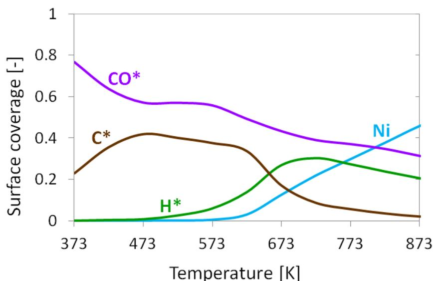
**Figure 5.8** Computed surface coverage of adsorbed species as function of the temperature for CO methanation at 1 bar, inlet gas composition of 2.04 vol.% CO and 7.0 vol.% H<sub>2</sub> in N<sub>2</sub> dilution; 1bar;  $T_{inlet}=373$  K; total flow rate of 4 SLPM.
