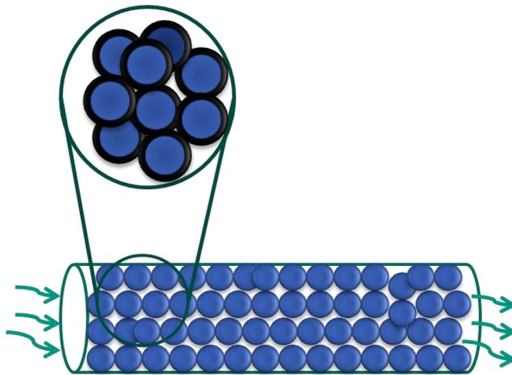
**Figure 2.4** Schematic diagram of a fixed bed reactor.
