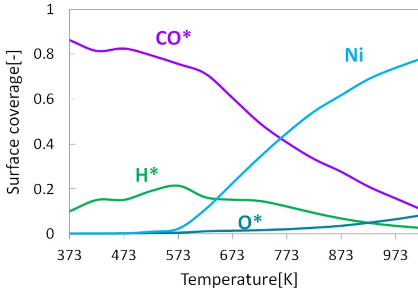
**Figure 4.18** Surface coverage as function of the temperature for preferential CO oxidation for an inlet mixture of 4.3 vol.% CO, 4.20 vol.% H<sub>2</sub>, 4.0 vol.% O<sub>2</sub> in N<sub>2</sub>; 1 bar;  $T_{inlet} = 373$  K; 4 SLPM.
