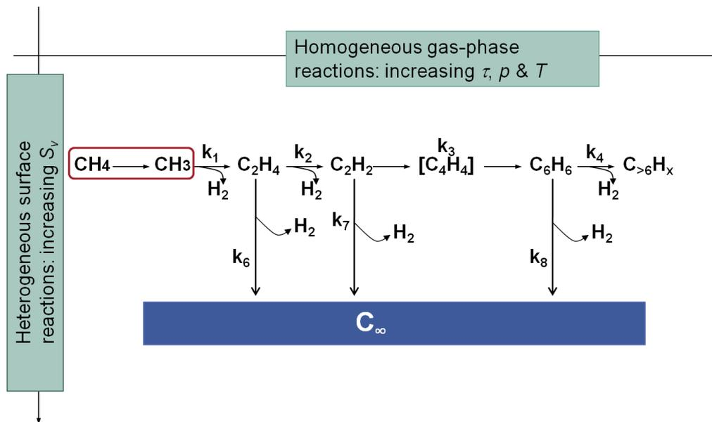
**Figure 4.60** Model of pyrocarbon deposition from methane [239, 240].
