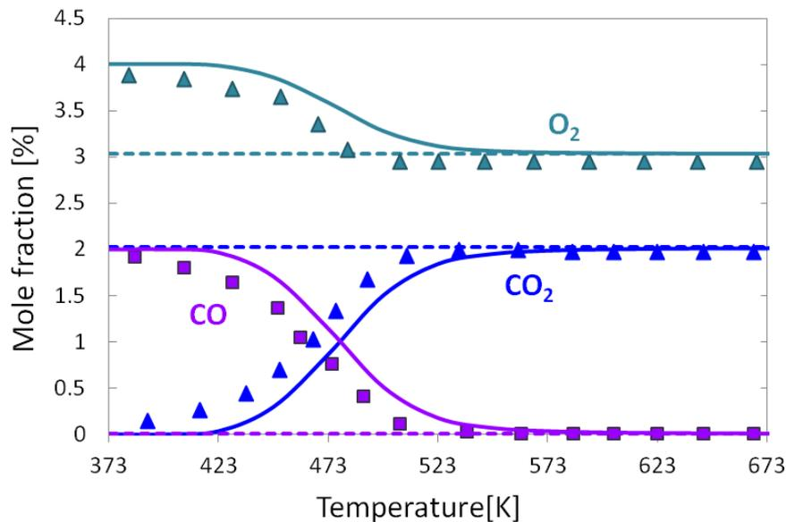
**Figure 4.6** Comparison of experimentally determined (symbols) and numerically predicted (lines) mol fractions as a function of the temperature for catalytic oxidation of CO in a fixed bed reactor;  $T_{inlet} = 373 \text{ K}$ ;  $CO/O_2 = 0.5$  (94 %  $N_2$ ) at 1bar; total flow rate of 2 SLPM; dashed lines = equilibrium composition at given temperature.
