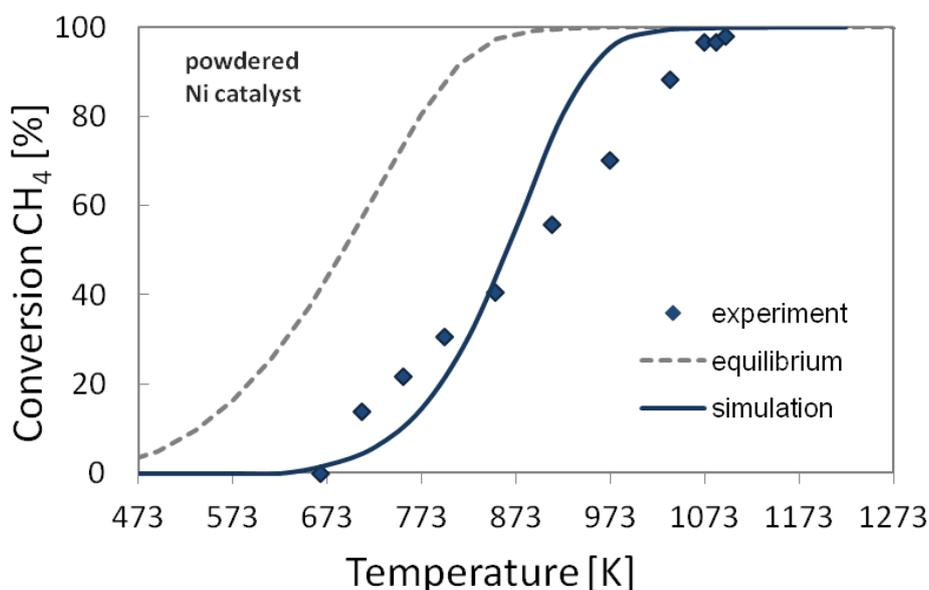
**Figure 4.53** Methane conversion as function of temperature over powdered Ni catalyst with Ni catalyst,  $S/C = 3$ ; 1 bar;  $T_{range} = 473\text{-}1273\text{ K}$ ;  $GHSV = 9443\text{ h}^{-1}$  experimental data taken from Ryu [221].
