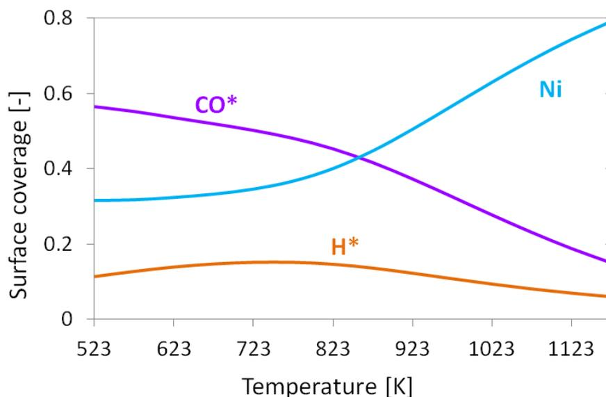
**Figure 4.39** Computed surface coverage of adsorbed species for methane dry reforming as a function of the temperature;  $CH_4/CO_2=1$  in  $N_2$ ; 1 bar;  $T_{inlet}=473$  K; total flow rate of 4 SLPM.
