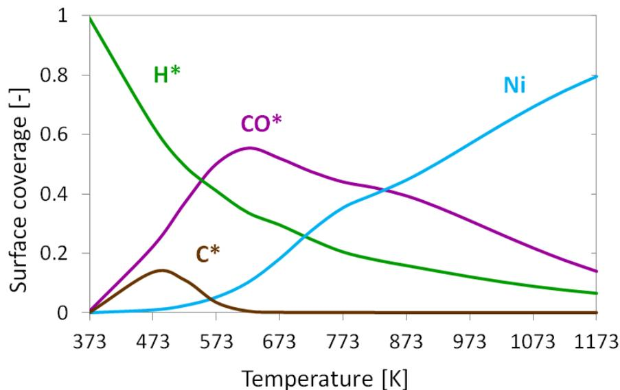
**Figure 4.42** Computed surface coverage of adsorbed species as function of the temperature for methane dry reforming with H<sub>2</sub> addition: inlet gas composition of 1.6 vol.% CH<sub>4</sub>, 2.1 vol.% CO<sub>2</sub>, 1.8 vol.% H<sub>2</sub> in N<sub>2</sub>; 1 bar;  $T_{inlet} = 373$  K; total flow rate 4 SLPM.
