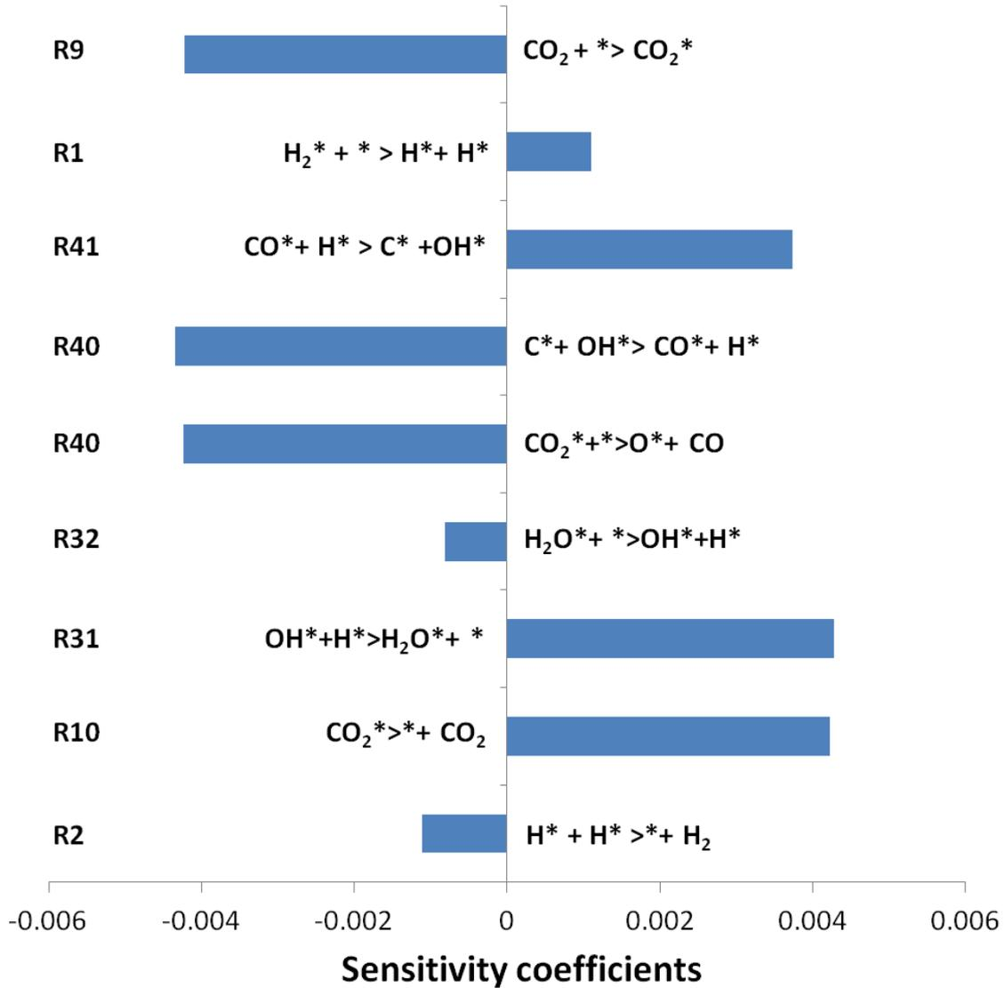
**Figure 4.43** Sensitivity analysis of absorbed C\* for dry reforming of methane with H<sub>2</sub> at 473 K, inlet gas composition of 1.6 vol.% CH<sub>4</sub>, 2.1 vol.% CO<sub>2</sub>, 1.8 vol.% H<sub>2</sub> in N<sub>2</sub>; 1 bar.
