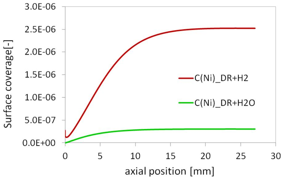
**Figure 4.46** Computed surface coverage for carbon along the catalytic bed for methane reforming with  $\text{CO}_2$  at 1123 K: **a)** comparison of methane dry reforming between the cases with  $\text{H}_2$  and steam addition, **b)** zoom-in of the surface coverage using  $\text{H}_2$  and  $\text{H}_2\text{O}$  as co-reactant.
