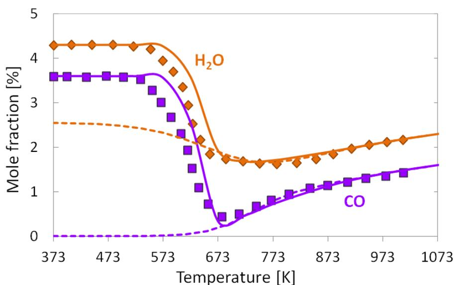
**Figure 5.2** Comparison of experimentally determined (symbols) and numerically predicted (lines) mole fractions as a function of temperature for WGS in a fixed bed reactor: **a)** CO and H<sub>2</sub>O; **b)** CO<sub>2</sub>, H<sub>2</sub>, and CH<sub>4</sub>, inlet gas composition of 3.6 vol.% CO, 4.3 vol. % H<sub>2</sub>O in N<sub>2</sub>; 1 bar;  $T_{inlet} = 373 \text{ K}$ ; 4 SLPM; dashed lines = equilibrium composition at given temperature.
