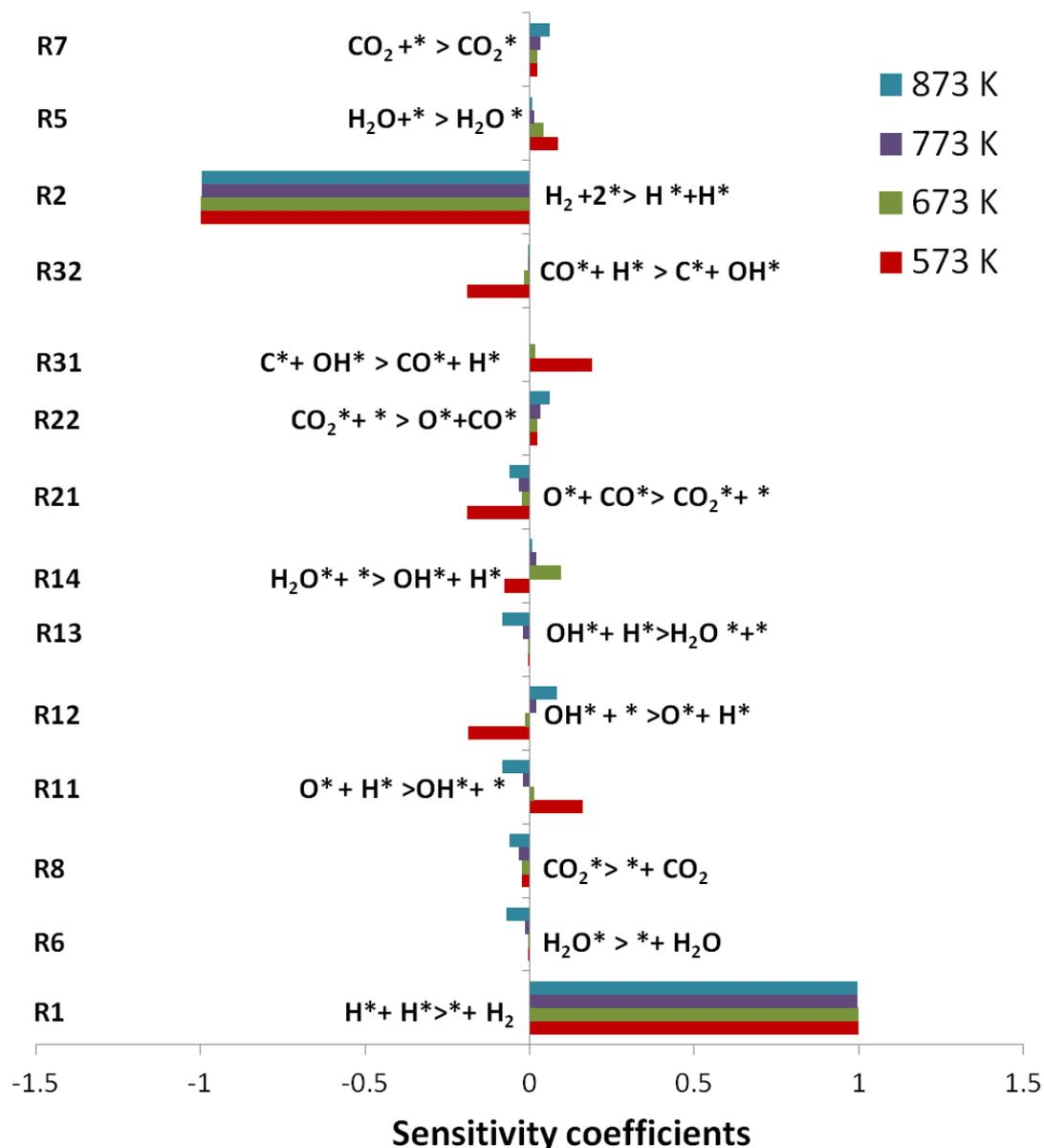
**Figure 4.20** Sensitivity analyses of  $H_2$  gas-phase concentration for WGS reaction at different temperature points. Inlet gas composition is chosen to be 3.6 vol. % CO and 4.3 vol. %  $H_2O$  in  $N_2$  dilution.
