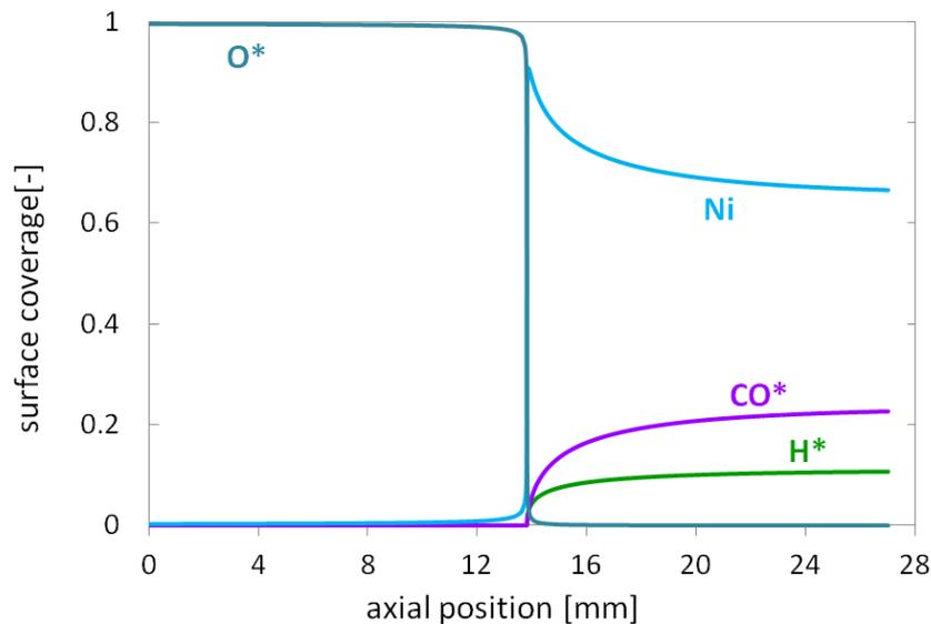
**Figure 4.33** Computed surface coverage of adsorbed species: **a)**  $\text{O}^*$ ,  $\text{CO}^*$ ,  $\text{H}^*$ ,  $\text{Ni}$ ; **b)**  $\text{OH}^*$ ,  $\text{H}_2\text{O}^*$ ,  $\text{CO}_2^*$ , and  $\text{C}^*$  along the catalytic bed after the ignition for partial oxidation of methane over nickel at 973 K (700 °C),  $\text{CH}_4/\text{O}_2=1.6$ .
