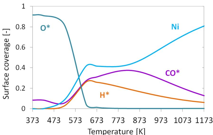
**Figure 4.45** Computed surface coverage of adsorbed species as function of the temperature for methane dry reforming with  $\text{H}_2\text{O}$  addition: 1.7 vol.%  $\text{CH}_4$ , 2.1 vol.%  $\text{CO}_2$ , 2.1 vol.%  $\text{H}_2\text{O}$  in  $\text{N}_2$ ; 1 bar;  $T_{\text{inlet}} = 373$  K; total flow rate of 4 SLPM.
