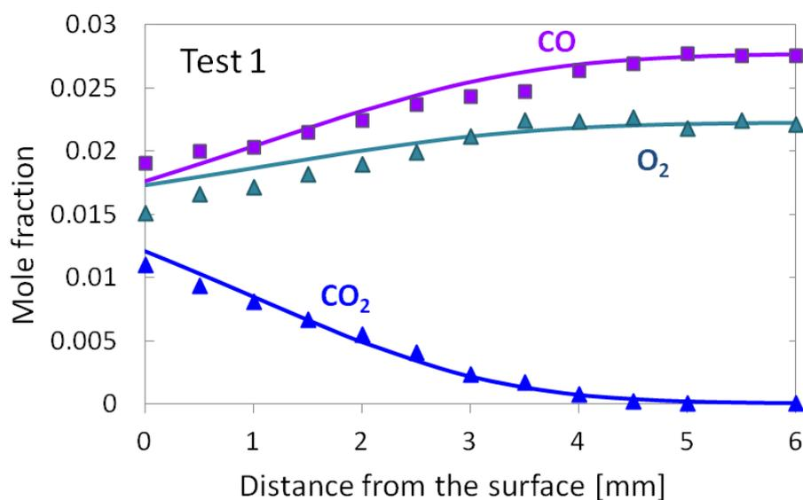
**Figure 4.10** Comparison of experimentally determined (symbols) and computed (lines) species profile in the stagnation-flow reactor for catalytic oxidation of CO at 573 K, 500 mbar, total flow rate of 15.5 SLPM.  $F_{cat/geo}=1.5$  is used in the numerical simulation.
