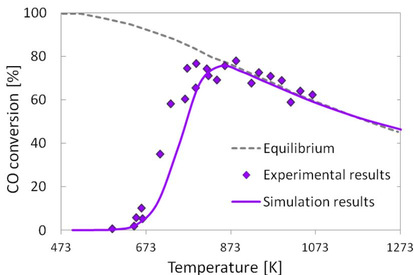
**Figure 4.29** CO conversion as function of the temperature in WGS on Ni supported on alumina foam monolith for a feed composition of 1/2/4 for  $\text{CO}/\text{H}_2/\text{H}_2\text{O}$  with 20 %  $\text{N}_2$  dilution.
