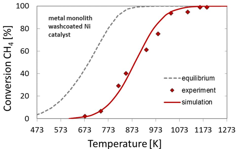
**Figure 4.52** Methane conversion as function of temperature over metal monolith wash-coated with Ni catalyst, S/C = 3; 1 bar;  $T_{\text{range}} = 400\text{-}1273$  K; GHSV=9443 h<sup>-1</sup> experimental data taken from Ryu [221].
