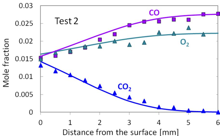
**Figure 4.11** Comparison of experimental (symbols) and computed (lines) species profile in the stagnation-flow reactor for catalytic oxidation of CO at 673 K; 500 mbar; total flow of 15.5 SLPM.  $F_{cat/geo}=1.5$  is used in the numerical simulations.
