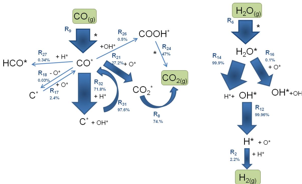
**Figure 4.21** Reaction flow analysis for WGS reaction on nickel at 673 K, 4 SLPM, inlet gas composition of 3.6 vol. % CO and 4.3 vol. % H<sub>2</sub>O in N<sub>2</sub> dilution.
