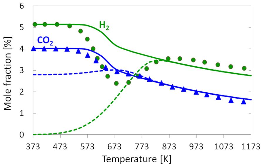
**Figure 4.27** Comparison of experimentally determined (symbols) and numerically predicted (lines) mole fractions as a function of temperature for R-WGS in a fixed bed reactor: **a)** CO<sub>2</sub> and H<sub>2</sub>; **b)** CO, H<sub>2</sub>O, and CH<sub>4</sub>; inlet gas composition of 4.0 vol% CO<sub>2</sub> and 5.1 vol% H<sub>2</sub> in N<sub>2</sub> dilution; 1bar;  $T_{inlet}=373$  K; 4SLPM; dashed lines =equilibrium composition at given temperature.
