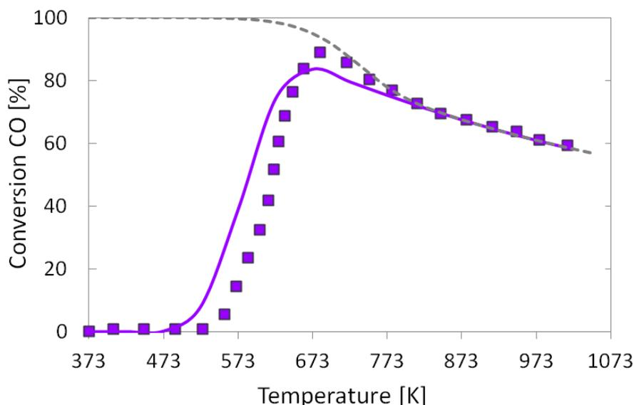
**Figure 4.23** CO conversion as a function of the temperature in water-gas shift reaction on Ni for an inlet gas composition of 3.6 vol. % CO, 4.3 vol. % H<sub>2</sub>O in N<sub>2</sub>; 1 bar;  $T_{inlet}$  = 373 K; 4 SLPM; symbols = experiment, lines = simulation, dashed lines = equilibrium composition at given temperature.
