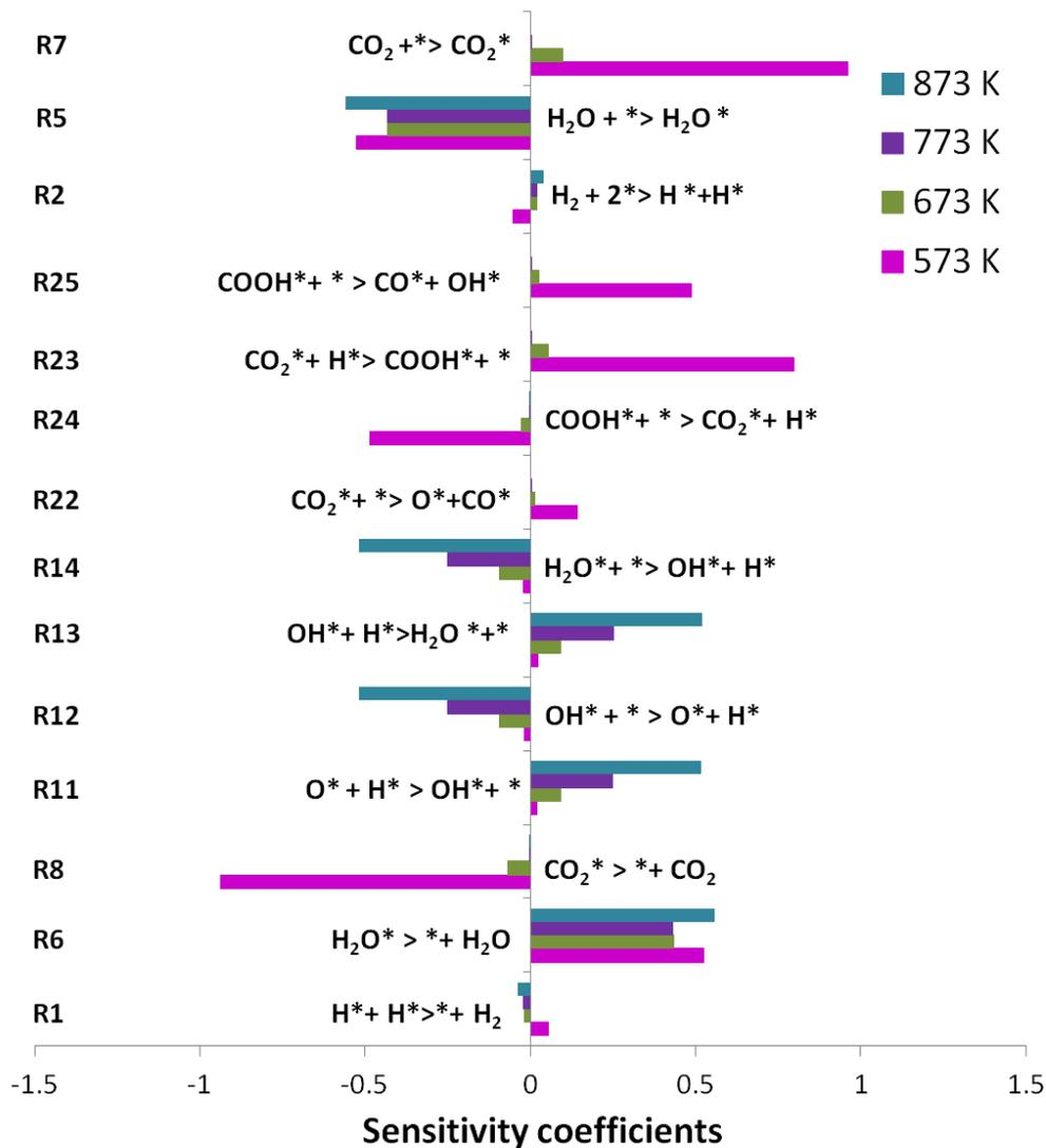
**Figure 4.26** Sensitivity analyses of H<sub>2</sub>O gas-phase concentration for R-WGS reaction at different temperature points. Inlet gas composition is chose to be 4.0 vol.% CO<sub>2</sub> and 5.1 vol.% H<sub>2</sub> in N<sub>2</sub> dilution.
