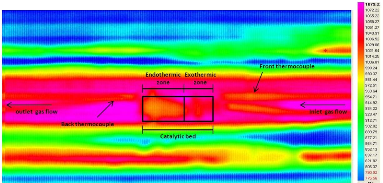
Figure 4.34 Infrared picture of the catalytic bed during partial oxidation of methane (CPOx).
