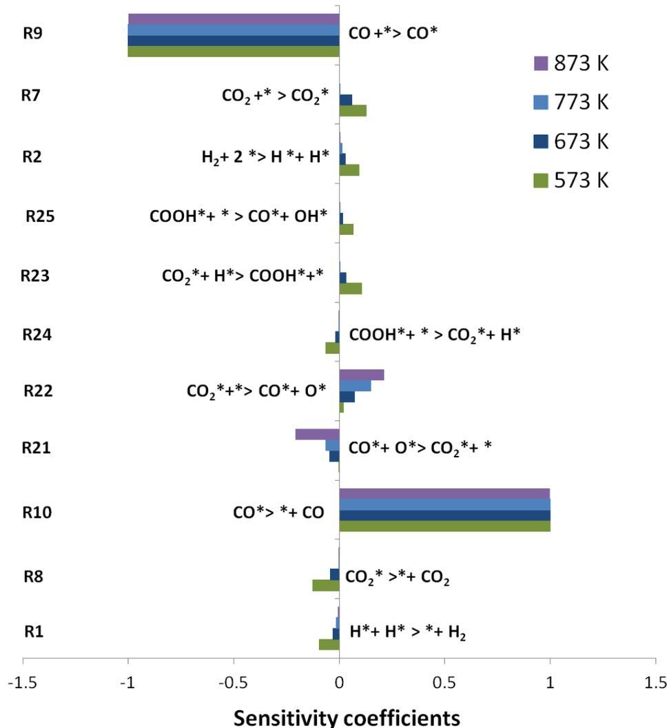
**Figure 4.25** Sensitivity analyses of CO gas-phase concentration for R-WGS reaction at different temperature points. Inlet gas composition is chosen to be 4.0 vol.%  $\text{CO}_2$  and 5.1 vol.%  $\text{H}_2$  in  $\text{N}_2$  dilution.
