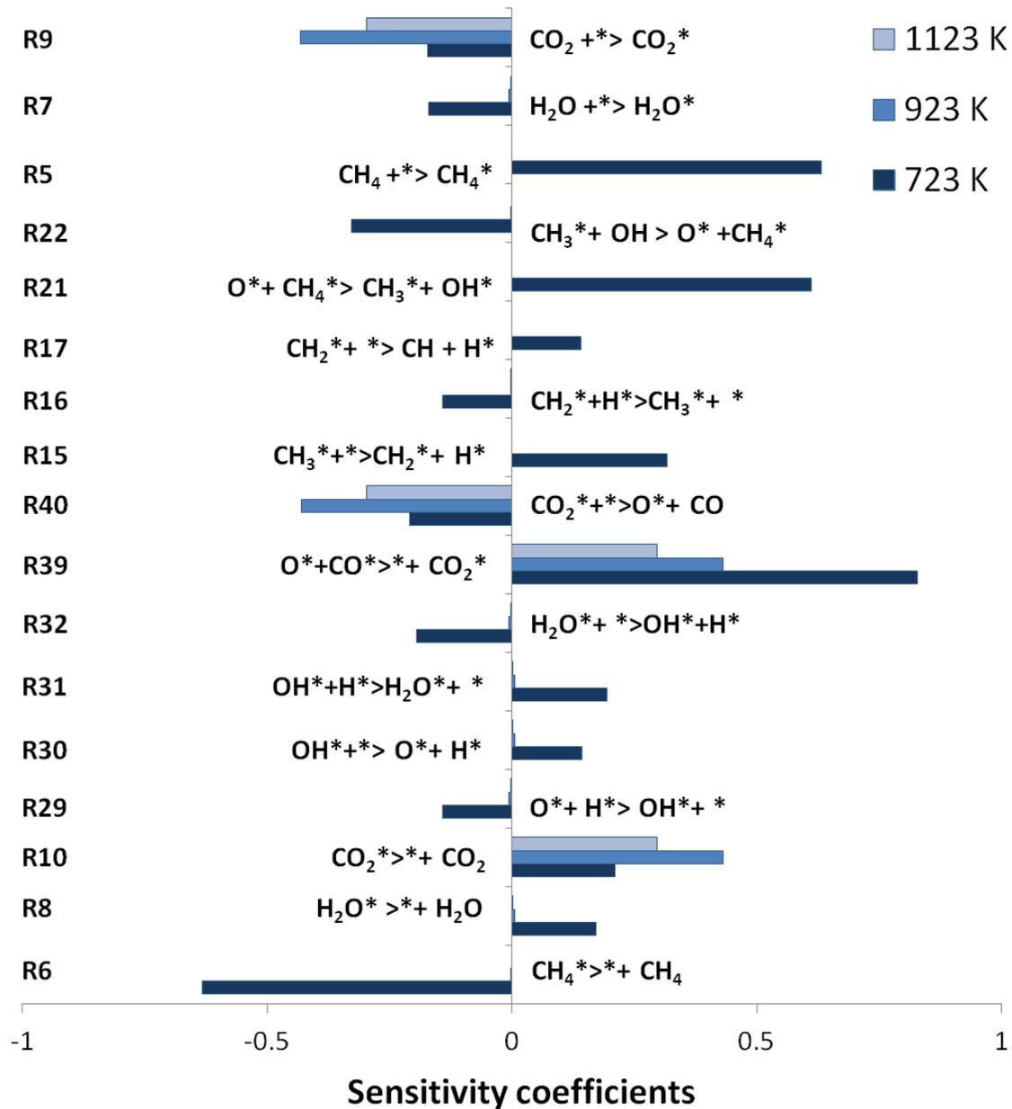
**Figure 4.37** Sensitivity analysis of  $\text{CO}_2$  gas phase concentration for steam reforming methane at different temperatures points for  $\text{CH}_4/\text{H}_2\text{O}= 0.8$  in  $\text{N}_2$  dilution.
