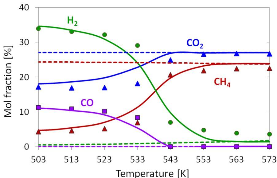
**Figure 5.10** Comparison of experimentally determined (symbols) and numerically predicted (lines) mole fractions as function of temperature for CO methanation: inlet gas composition of 11.75 vol.% CO, 35.52 vol.% H<sub>2</sub>, 0.0059 vol.% O<sub>2</sub>, 4.06 vol.% CH<sub>4</sub> and 17.56 vol.% CO<sub>2</sub> in N<sub>2</sub> dilution; 1.8bar;  $T_{inlet}=453$  K;  $\tau_{mod,CO}=76$  kg\*s/mol; dashed lines =equilibrium composition at given temperature.
