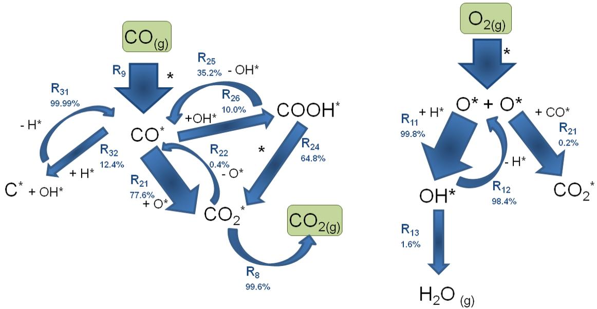
**Figure 4.16** Reaction flow analysis for CO preferential oxidation on nickel at 573 K, total flow rate of 2 SLPM, inlet gas composition of 2.22 vol.% CO, 1.90 vol.% H<sub>2</sub>, 4.0 vol% O<sub>2</sub> in N<sub>2</sub> (94 % N<sub>2</sub>), 1bar.
