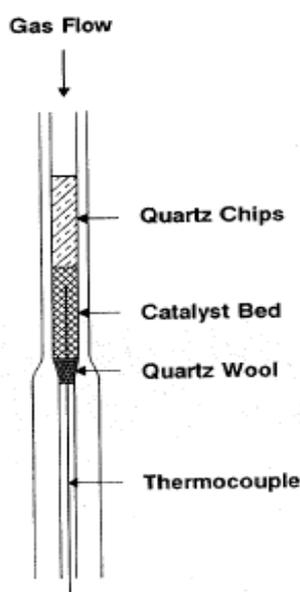
**Figure 4.47** Schematic representation of the continuous-flow reactor [16].
