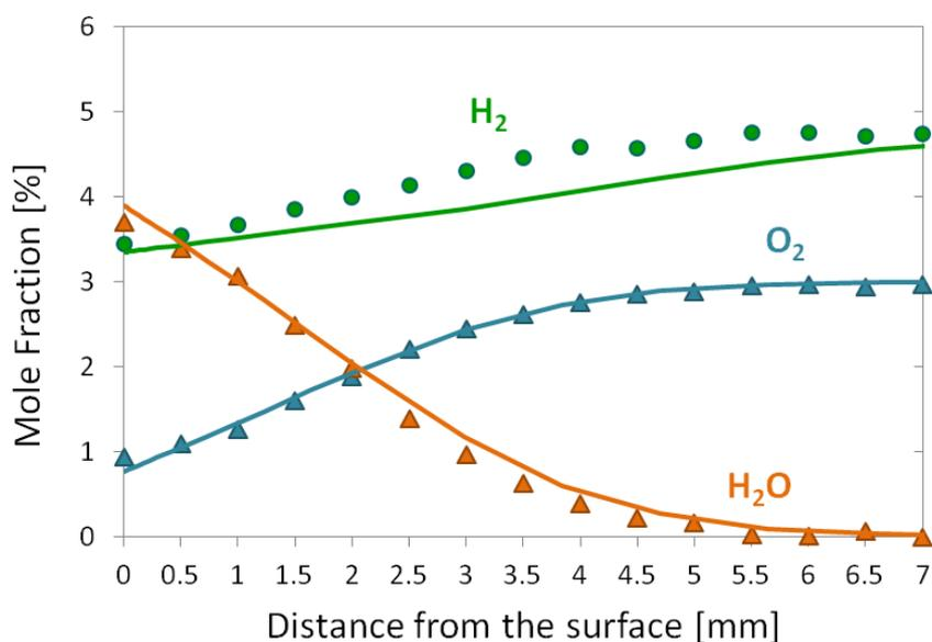
**Figure 4.5** Comparison of experimentally determined (symbols) and numerically predicted (lines) mole fractions as function of the temperature for catalytic oxidation of H<sub>2</sub> in a stagnation-flow reactor at 623 K; H<sub>2</sub>/O<sub>2</sub>=1.65 (92 % Ar) at 500 mbar; total flow rate of 15 SLPM.
