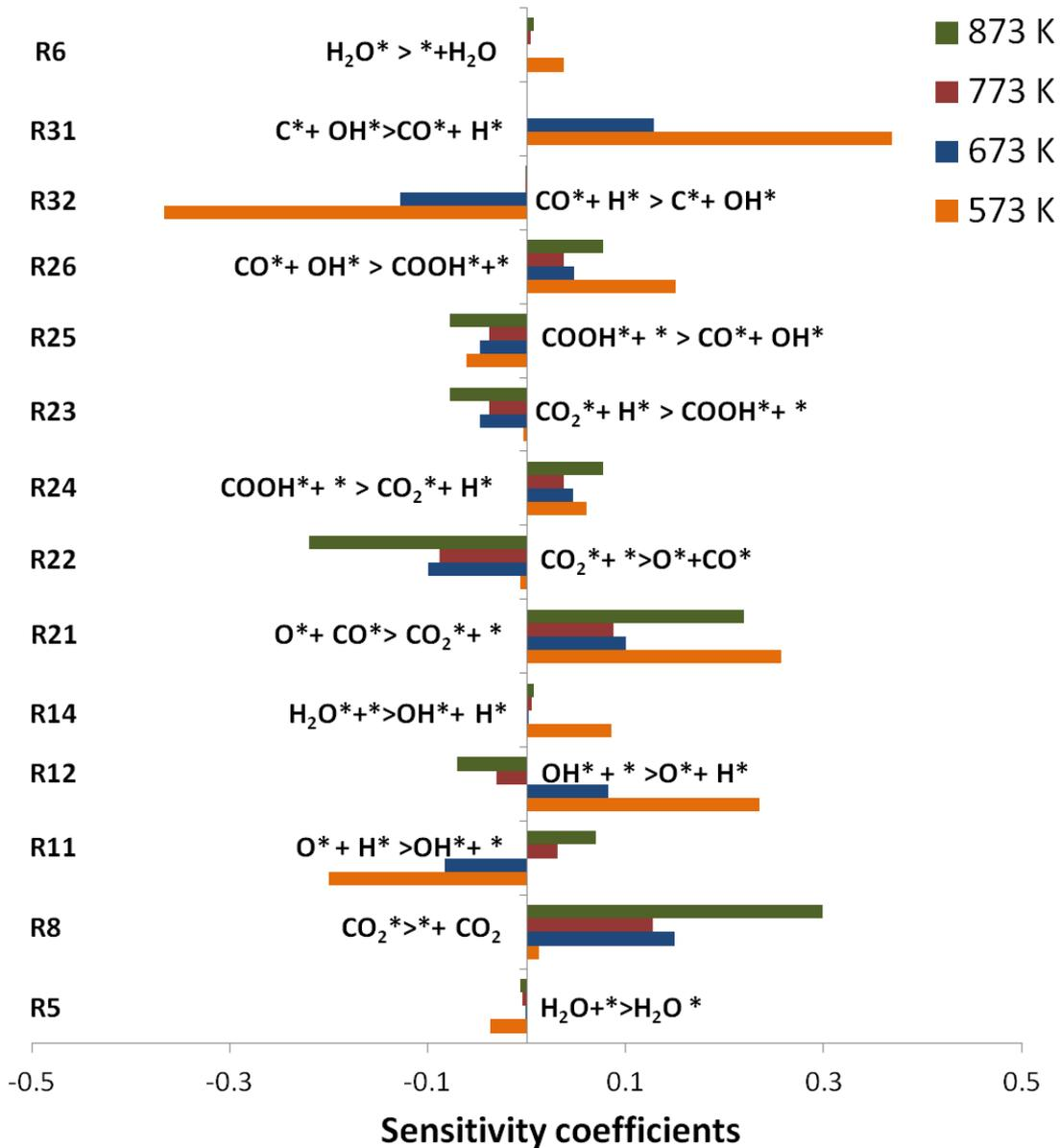
**Figure 4.19** Sensitivity analyses of  $\text{CO}_2$  gas-phase concentration for WGS reaction at different temperature points. Inlet mole composition is chosen to be 3.6 vol.% CO and 4.3 vol.%  $\text{H}_2\text{O}$  in  $\text{N}_2$  dilution.
