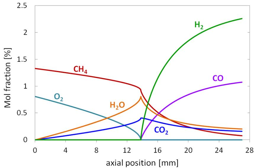
**Figure 4.32** Computed mole fraction of the gas-phase species:  $\text{O}_2$ ,  $\text{CH}_4$ ,  $\text{H}_2$ ,  $\text{H}_2\text{O}$ ,  $\text{CO}$  and  $\text{CO}_2$  along the catalytic bed after the ignition for partial oxidation of methane over nickel at 973 K,  $\text{CH}_4/\text{O}_2=1.6$ .
