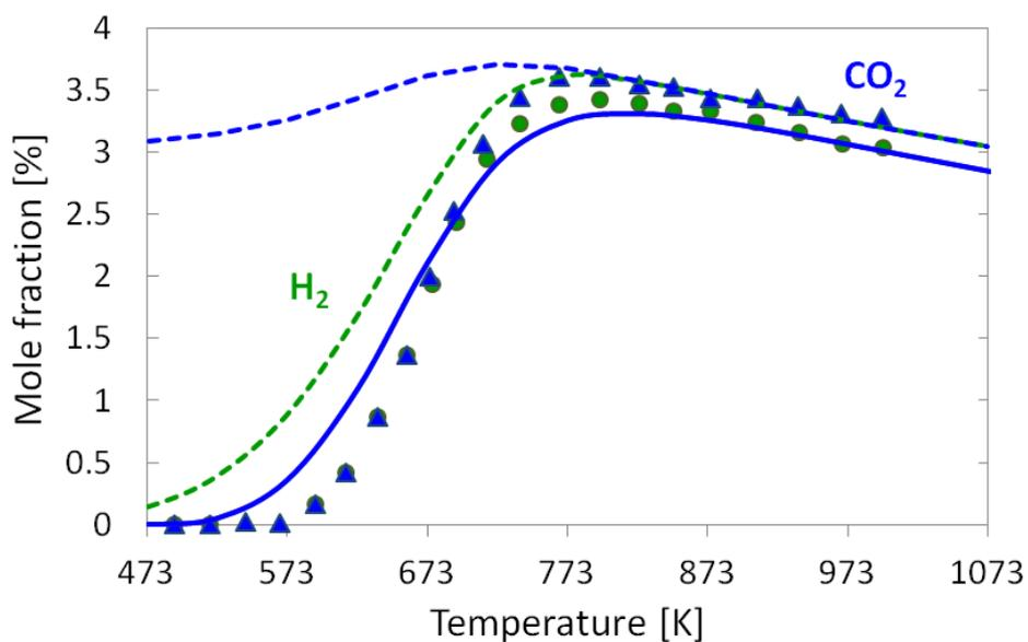
**Figure 4.24** Comparison of experimentally determined (symbols) and numerically predicted (lines) mole fractions as a function of temperature for WGS in a fixed reactor: **a)**  $CO$  and  $H_2O$ ; **b)**  $CO_2$ ,  $H_2$ , inlet gas composition of 4.0 vol. %  $CO$ , 12.7 vol.%  $H_2O$  in  $N_2$ ; 1 bar;  $T_{inlet}= 373$  K, 4 SLPM, dashed lines = equilibrium composition at given temperature.
