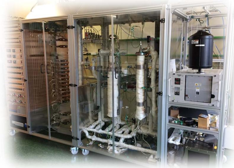
Tests of catalyst coated honeycombs
